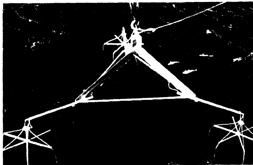
Figure E-2. Electrofishing gear tested for harvesting northern squawfish at Bonneville Dam First Powerhouse, summer 1991. Top, wingwall electrode array; middle, piernose electrode array; bottom, portable electrode array.
